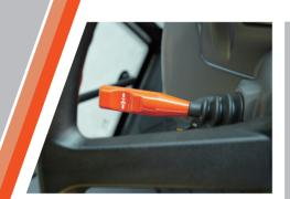
Power Shuttle Lever (Power Shuttle Models)
